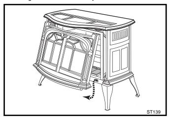
Fig. 5 Remove the front plate.
